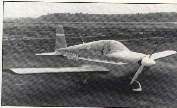
In 1972 Grumman American introduced the AA-1B Trainer, which was powered by a 108-hp Lycoming O-235-C2C engine. The only real difference between it and its predecessor (the A-model Trainer) was an increase of the maximum gross weight from 1500 to 1560 pounds.
