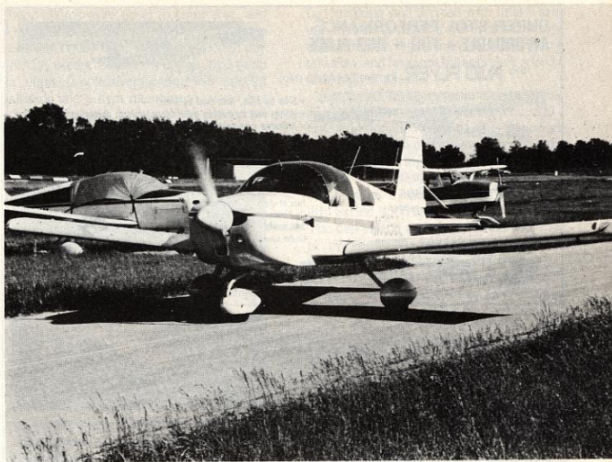
Taxiing calls for operational brakes and a toe-steering technique due to the responsive, castering nosewheel.
