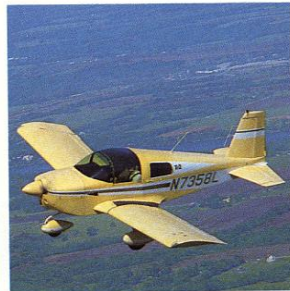
The Tr2's stubby, 25-foot wingspan earned the ship a reputation for lethargic takeoffs and hot landings.
