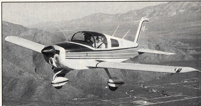
The AA-1 series is renowned for its 100+ knot cruise speeds. It is equally infamous for its lackluster climb performance, especially when operating with full fuel and passengers from locations with high temperatures and high-density altitude.
